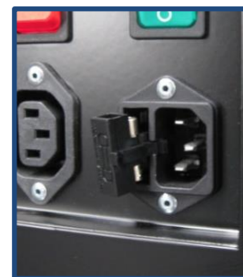
Picture 3. Glass fuse in connector
